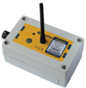
TGRF-3201: Tinytag Radio temperature logger for PT1000 probe (-200 to +200°C) A single channel radio temperature logger for use with a PT1000 probe, for monitoring over a wide range of temperatures.
