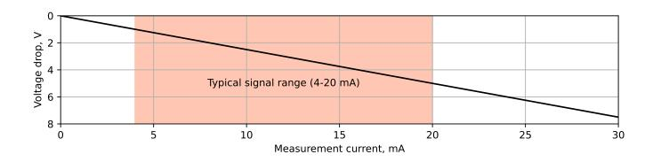
Please consult the documentation of the external  $4-20\,\text{mA}$  signal source to verify that a load of  $250\,\Omega$  and the associated voltage drop are applicable to the particular device. Failure to observe these constraints might result in unstable operation or damage to the  $4-20\,\text{mA}$  signal source device.
